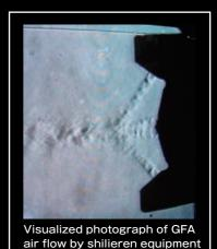
Painting conditions Paint: metal-tinged paint Paint output: 70ml/min Number of gun passes: 3times Paint film thickness: 6µ
