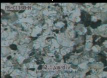
Metal flakes are floating and coloring pigments are coagulated.
