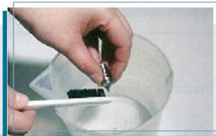
7. Remove the fluid nozzle with a 17mm box end wrench and wash it with the exclusive brush
