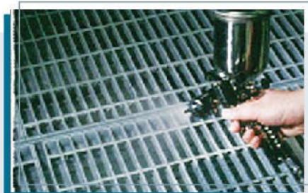
4. Spray the thinner in front of a spraying booth. Repeat about 3 times.
