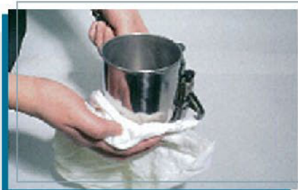
5. Clean the outside of the cup and the spray gun with waste clothes moistened with cleaning thinner
