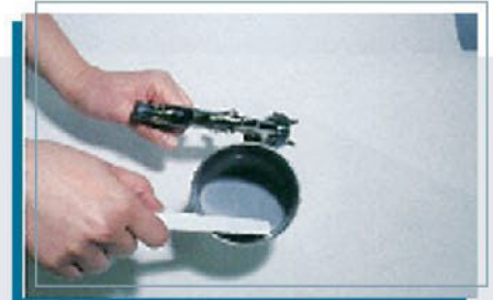
3. Wash cup's inside with the exclusive brush that enclosed with the spray gun
