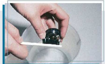
6. Remove the air cap and wash it with the exclusive brush
